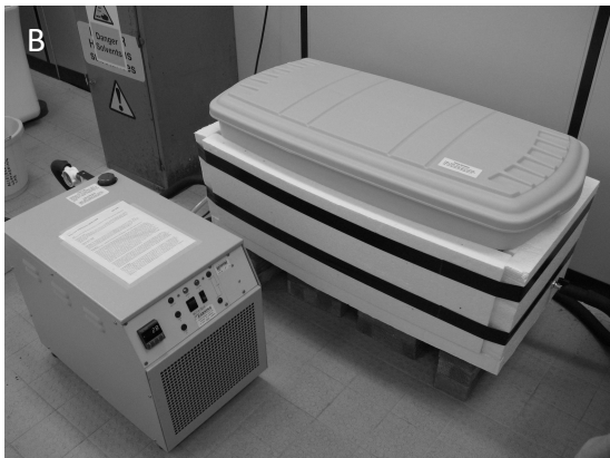
Figure 3.2: Warm water submersion model. A: A diagrammatic representation of the warm water submersion apparatus. Tanks a: bovine bone submerged in distilled water, b: bovine bone submerged in synthetic seawater and c: human bone submerged in synthetic seawater. B: Photograph of the closed tank with surrounding insulation. C: view of the arrangement of sample tanks within the main tank.
