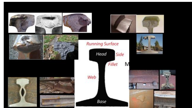
Fig. 1. Railway rail damages are mainly divided into four categories: transverse damages, longitudinal damages, web damages, miscellaneous damages.
