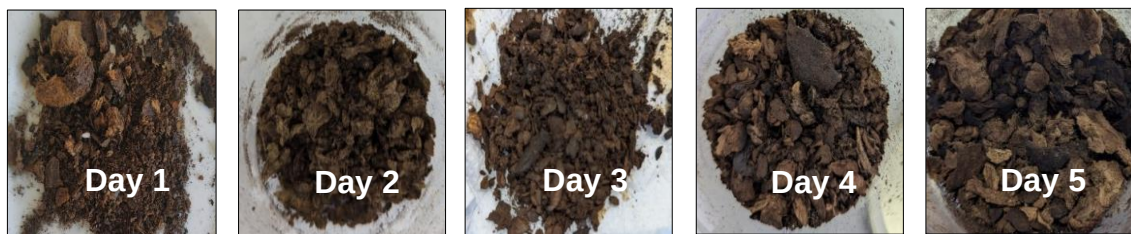
Figure 4-7 The physical appearance of biochar samples collected over five days at a torrefaction temperature of 250°C and a rotation speed of 0.083 RPM
