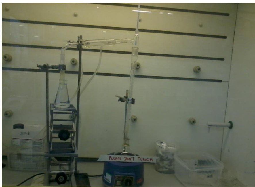
Figure 3-3: Fractional distillation of crude oil under laboratory conditions
