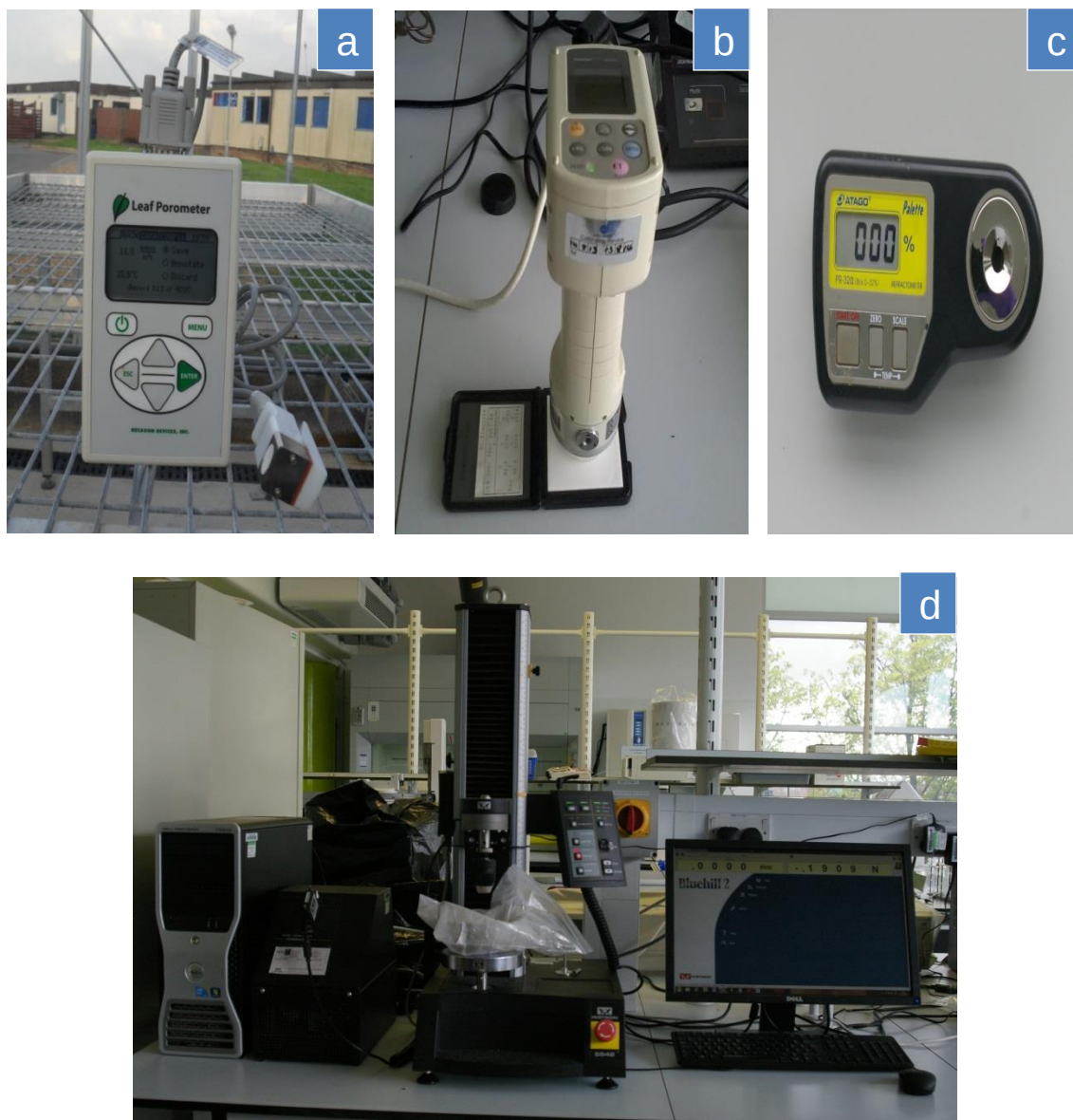
Figure 3-14: Growth and postharvest parameters measuring instruments: (a) the leaf porometer, (b) the chroma meter, (c) the palette digital refractometer, and (d) the Instron Bluehill® 2 system
