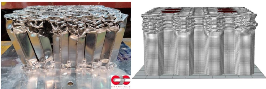
Fig. 19 Experimental and FEM results after impact test
