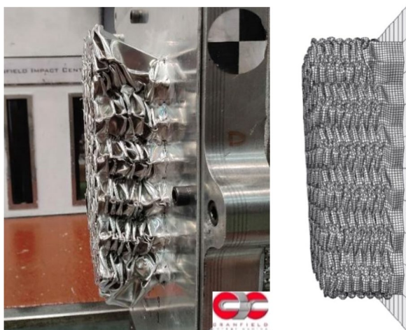
Fig. 17 Comparison between empty FEM and empty dynamic test specimen
