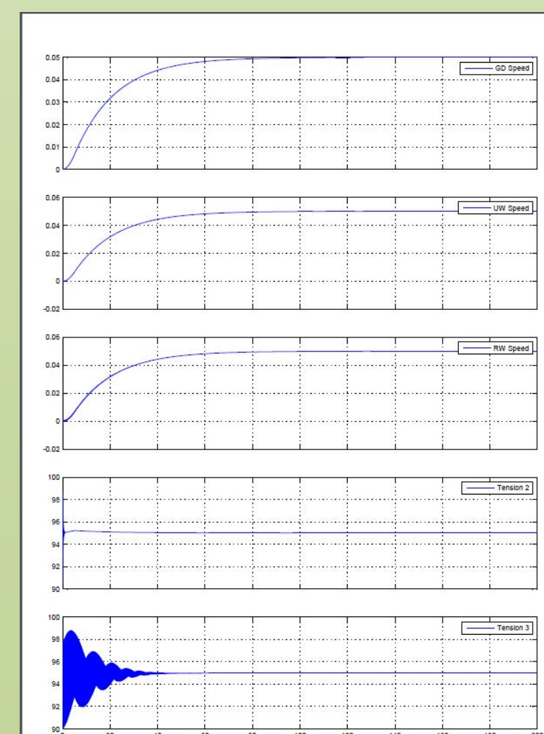
Figure 4 (a): Roller speeds and webspan tension with the GD controller proportional gain K_p = 1
