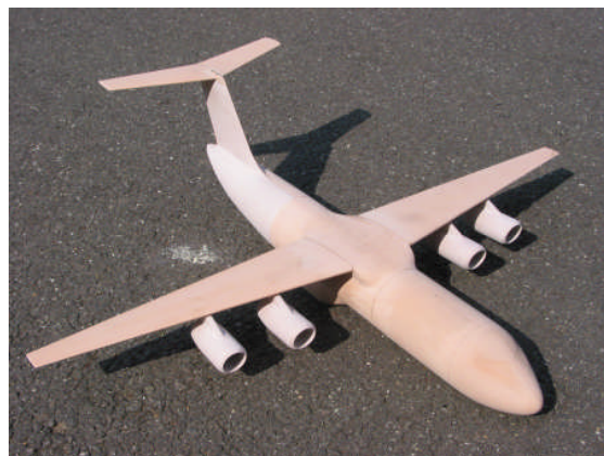
Figure 6 – Completed F-02 Wind Tunnel Model (Before Painting)
