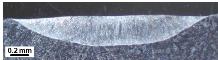
Figure 6-31 The width and cross-sectional profile of the bead on plate processing at 75 mm/s of TS, 3.0 mm of BD, and 2.79 kW of LP with a speed ratio of 1.25.
