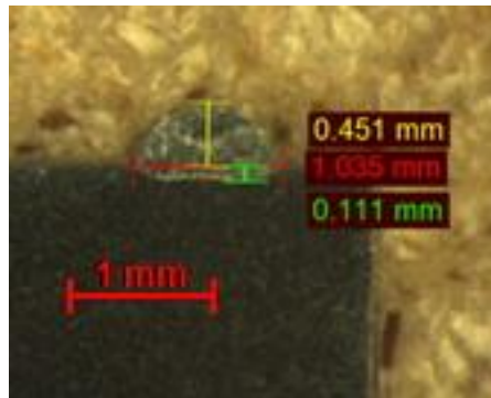
Figure 4-33 Image of the conduction mode profile of the cross-section of the deposit within group G4-1 (WFS/TS: 1.33).
