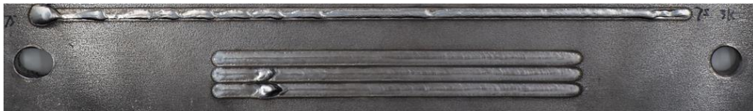
Figure 6-37 Image of three autogenous laser welds running before the experiments out of the experimental region.
