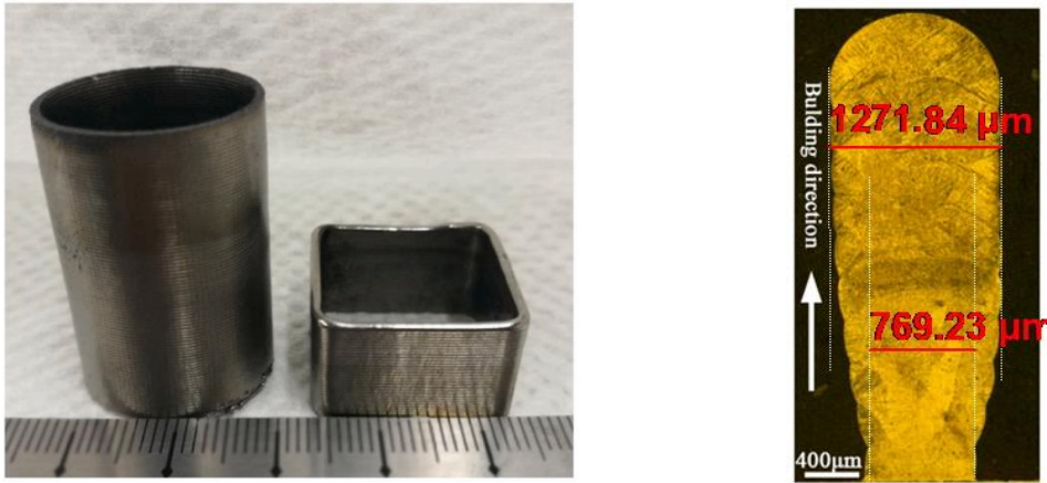
Figure 5-34 (a) Surface condition of Ti6Al4V thin-wall structures, and (b) cross-sectional profile and dimensions of Ti6Al4V thin wall (X. Ding, Ma, et al., 2022).
