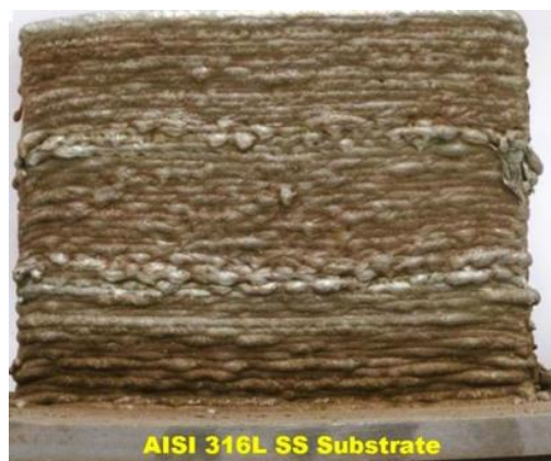
Figure 5-39 Surface roughness condition of AISI 316L SS fabricated by cold metal transfer WAAM process (Kumar et al., 2024).
