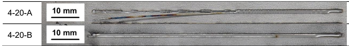
Figure 4-29 Images of the top-view appearance of the wire deviating from the original position of deposits 4-20-A and B.
