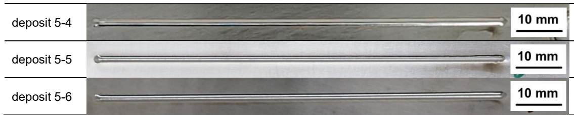
Figure 5-11 Images of the overall top view of bead on plate at 1.50 mm to 2.00 mm BD, (a) deposit 5-4, (b) deposit 5-5, and (c) deposit 5-6. (WFS = 5; TS = 5). Unit: mm/s.
