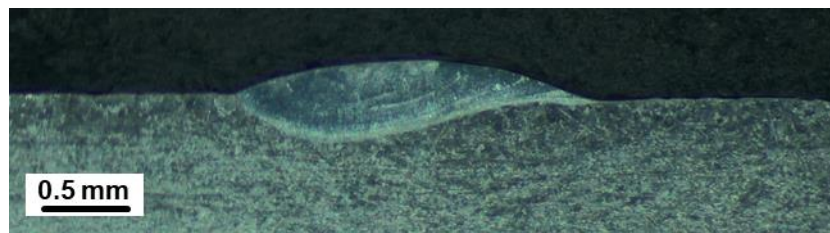
Figure 6-30 The width and cross-sectional profile of the bead on plate processing at 75 mm/s of TS, 3.0 mm of BD, and 2.79 kW of LP with a speed ratio of 1.00.
