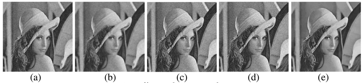
Fig. 2 Visual comparison of denoising results on the Lena image corrupted by additive white Gaussian noise with standard deviation 50. a Wiener filter [16] (PSNR = 22.95 dB; SSIM = 0.456); b Bilateral filter [38] (PSNR = 24.63 dB; SSIM = 0.589); c PCA method [9] (PSNR = 26.68 dB; SSIM = 0.596); d Wavelet transform [40] (PSNR = 21.74 dB; SSIM = 0.316); e Collaborative filtering: BM3D [55] (PSNR = 31.26 dB; SSIM = 0.845)
