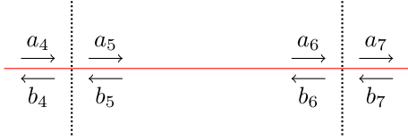
Figure 2: Schematic of the electric field components across two plane parallel interfaces.
