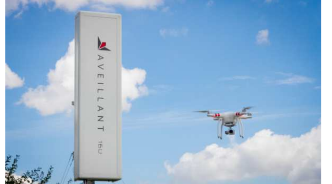
Fig 1. Aveillant Gamekeeper 16U holographic radar
