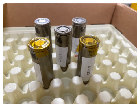
Figure 2. Samsung NCA cylindrical cells.
