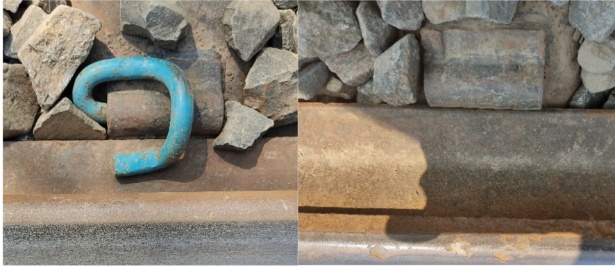
Fig. 2. Correct clip v broken clip.
