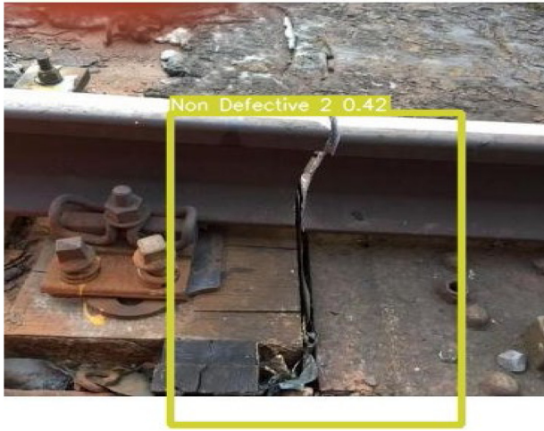
Fig. 14. Defective 2 wrongly classified as non-defective 2.
