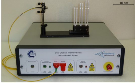
Fig. 1. The optical setup is sketched in (a), with the light leaving the interrogation unit guided by a fibre collimator/focuser to and from an arrangement of three different tuning forks that have small PMMA cuboids attached to their prongs, where the PMMA surface reflections that are evaluated are labelled. (b) shows a photograph of the fully-enclosed interrogation unit and the tuning fork arrangement.
