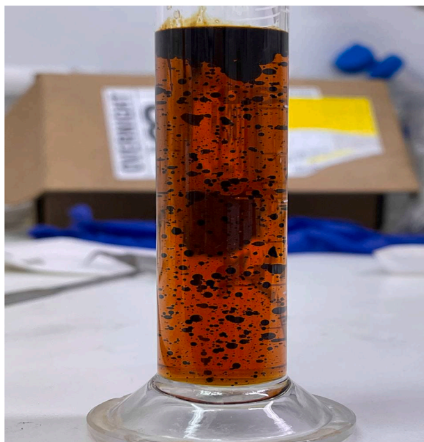
Fig. 10. Biooil from test 6 containing high water content with solubilizing acids, alcohols and ketones from carbohydrate decomposition [66].
