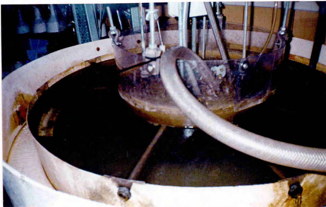
Plate 1. Pilot Clarifier with Un-Ozonated Water with Pass 100 at an Optimum Dose of 3.5 mg/l.
