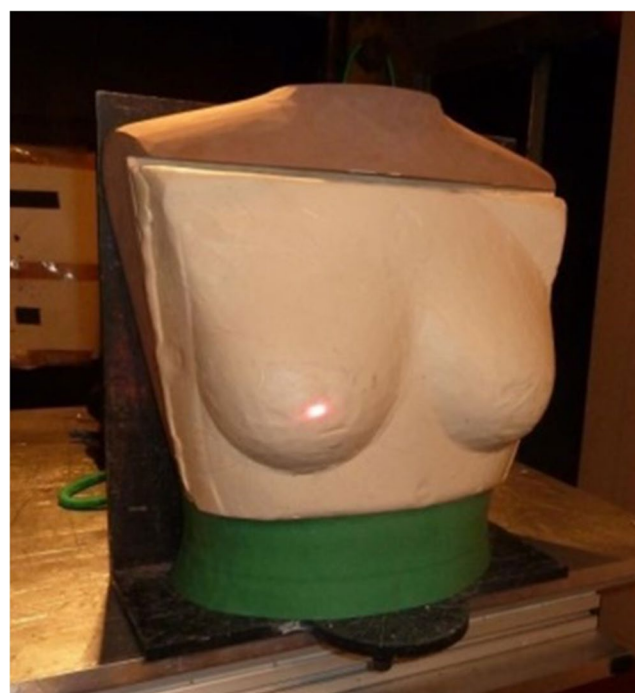
Fig. 2 Example female test form as specified in home office body armour standard 2017 (image produced by author)
