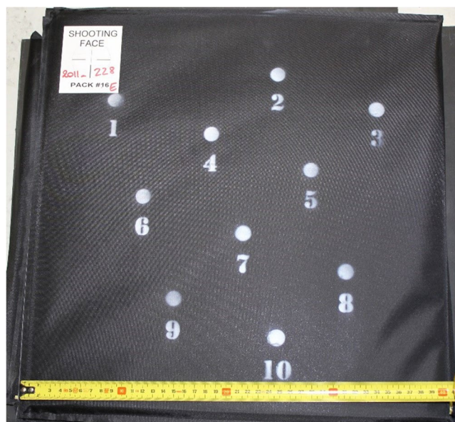
Fig. 3 Shot location marked on test panel
