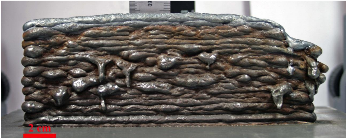
(a) torch shielding only (wall size: 180×68×9.8mm)
