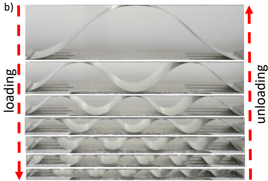
Figure 5-5: a) Front view of initial arc-shaped metallic glass foil; b) harmonic undulatory behaviour response of arc-shaped metallic glass foil.
