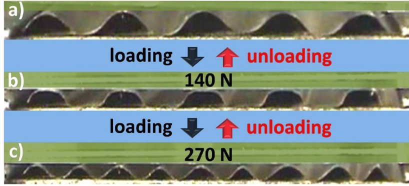
Figure 2-27. Front-view snapshots of the shaped MG foil: a) Free-standing pre-shaped MG foil; (b) elastic deformation at the maximum load when still functioning as a conventional wave spring; (c) the undulatory behaviour in which further loading leads to elastic multiplication of the number of arcs in the waveform and to an increase in the load capacity [118].
