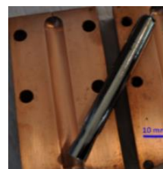
Fig. 1. MG rod ( \text{Zr}_{55}\text{Cu}_{30}\text{Ni}_{15}\text{Al}_{10} , about \varnothing 10 mm, 100 mm long) produced at Cranfield University by tilt casting into a copper mould.
