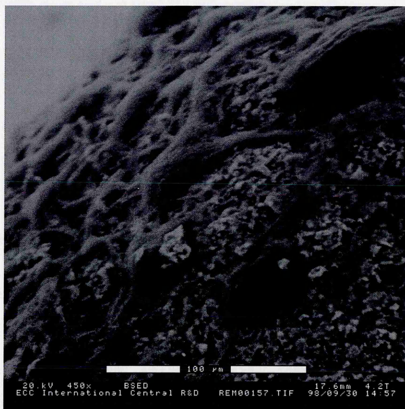
Figure 9.11: Micrograph showing the biofilm spreading across the surface (BSED)
