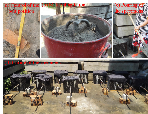
Fig. 1. Pouring and curing of pulling specimens.
