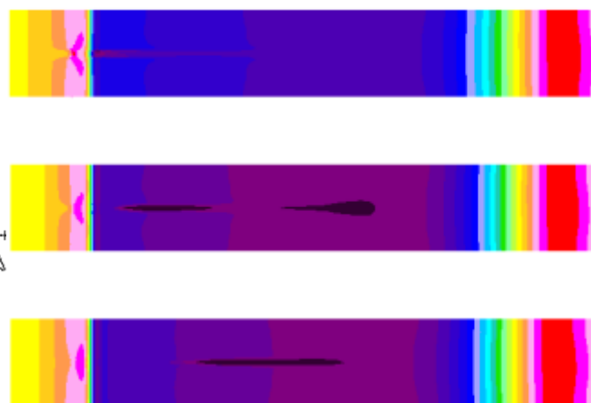
Fig. 4. Shock wave and separation produced in PREPHA program [11]
