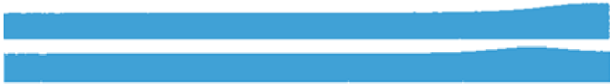
Figure 10: shows a single wave generated case for a largewater constrained tank illustrating velocity difference between a non-updated (top picture) and 50 timestep density updated (bottom picture) at time 22s
