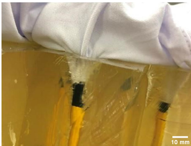
FIGURE 9 Illustrating pull-in of T-shirt into the wound tract by bolt, from series 2.
