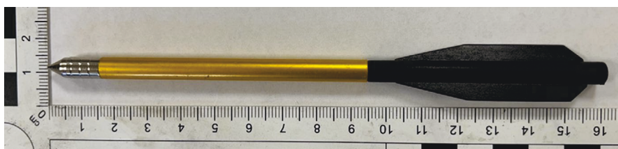
FIGURE 1 16.5 cm/ 6.5" field-tipped crossbow bolt used in experiment.
