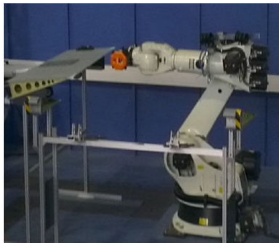
Figure 1: A metrology assisted demonstrator cell using a high payload industrial robot
