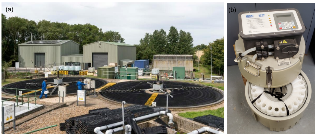
Figure 3.1 (a) Cranfield University wastewater sample collection point (b) ISCO 3700 sampler and 250 mL collection bottles for sampler
