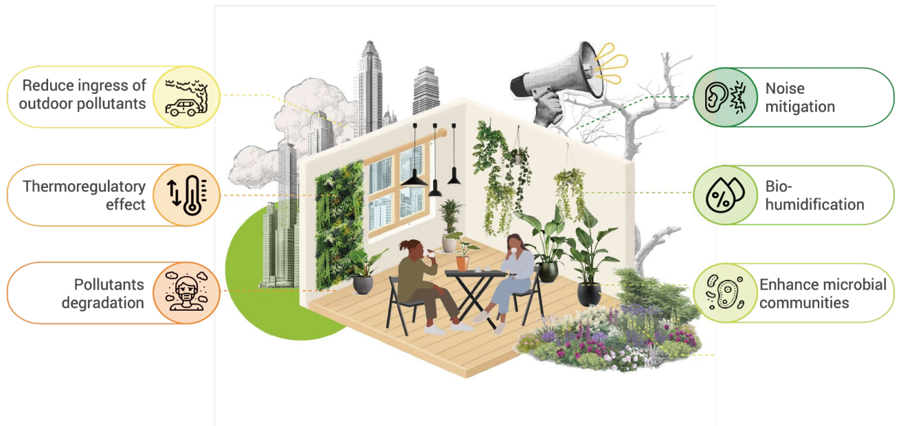
Figure 3. Pathways of iGI influencing IEQ, including effects on pollutants, microclimate, temperature, humidity, noise, stress, and microbial communities (Source: authors' original illustration).
