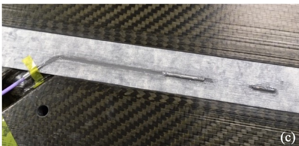
Figure 8.8: Pictures showing the manufacturing process to embed the optical fibres. (a) process involves the resin applied in the groove (b), the resin applied to the optical fibre (c) and the optical fibre placed in the groove with the resin filled flush.
