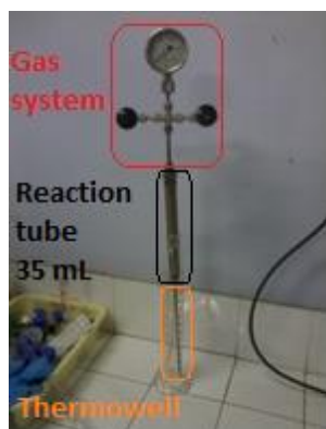
Figure 12 – Tubular system with pressure gauge and valves
