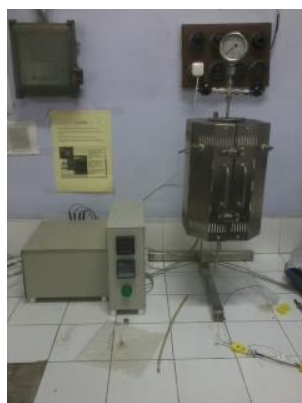
Figure 13 – HTL reactor with temperature controller
