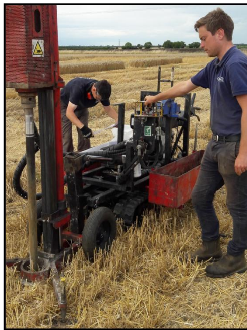
Figure 5-1 Clarke operating a smaller diameter version of the soil corer rig in 2017 on a plot experiment in Cambridge
