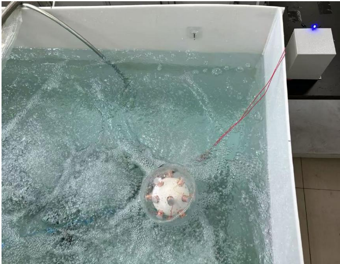
Fig.S21 C-TENG's motion form in the aeration tank.
