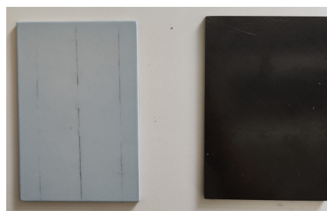
Figure 1. Photographs of the CFRP specimen: (left) front surface and (right) back surface, where the transducer was bonded for ultrasonic excitation; this surface also faced the infrared camera during testing.
