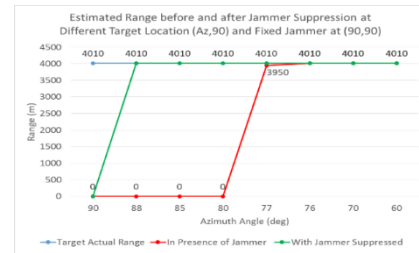
Figure 12 True and estimated range for Target at different azimuth with and without Jammer suppression.
