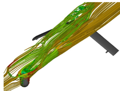
(b) Streamlines on modified geometry (flow spread indicates blanking phenomenon)
