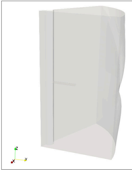
FIGURE 17: FIGURE DEPICTS THE QUARTER DOMAIN OF THE APPLICATION TO ROTATING WINGS (CARADONNA AND TUNG ROTOR) CASE.
