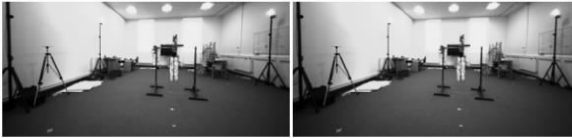
Figure 2.7: Left and right undistorted and stereo rectified images acquired in our laboratory at Cranfield University. The images show a mock-up of the Envisat satellite.
