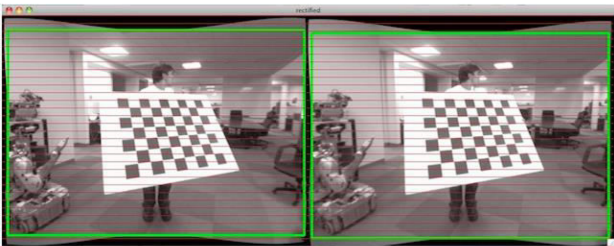
Figure 3.12: Pair of stereo rectified images. Horizontal lines match corresponding features [39].
