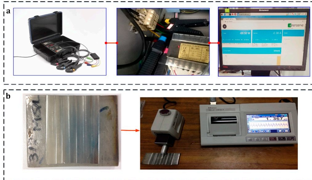
Figure 4. Experimental equipment used, showing: (a) power measurement using a Portable Power Cell PPC-3 (b) surface roughness measurement.
