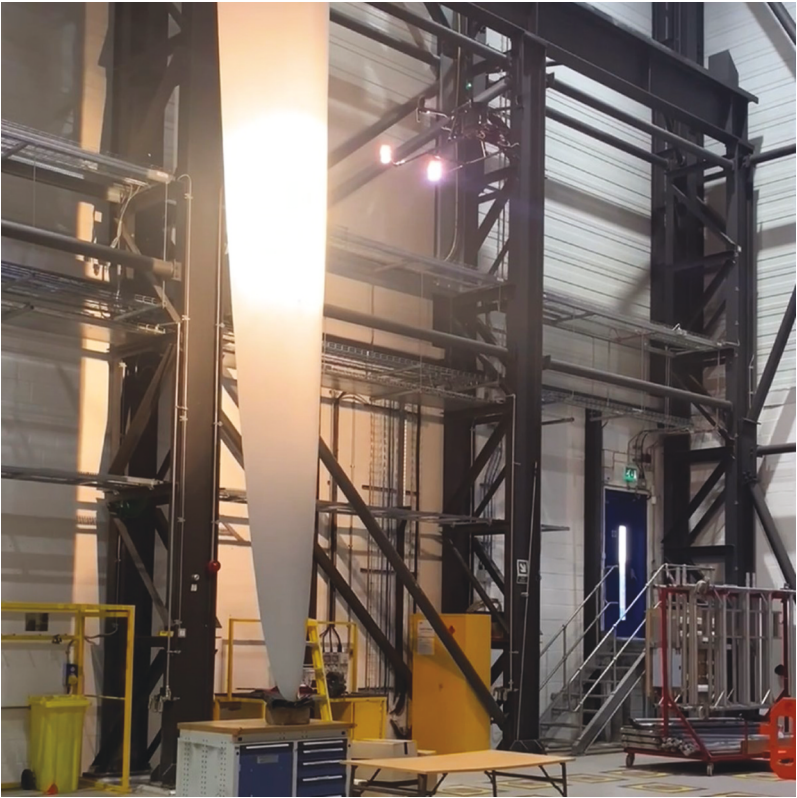
Figure 34. The active IR drone platform inspecting a composite wind turbine blade.
