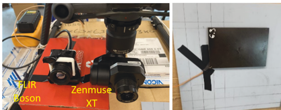
Figure 21. (A) An image of the FLIR Boson and the Zenmuse XT. (B) An image of the composite sample.
