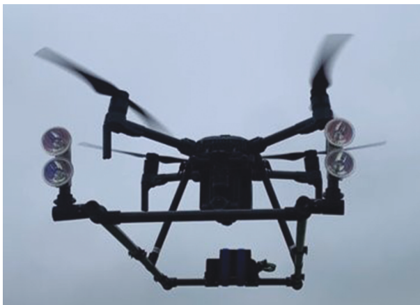
Figure 1. UAV with active thermography capabilities.
