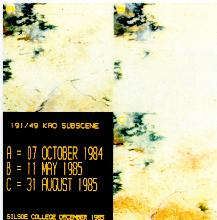
Plate 1. Band 4, 2, 1 Red, Green, Blue Landsat MSS false colour composites of the Kao study area from October 1984, May 1985 and August 1985. The full resolution image for 7th October 1985 can be seen in plate 6a.
