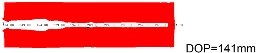
Figure 13. Depth of penetration for 32 mm shaped Charges.
