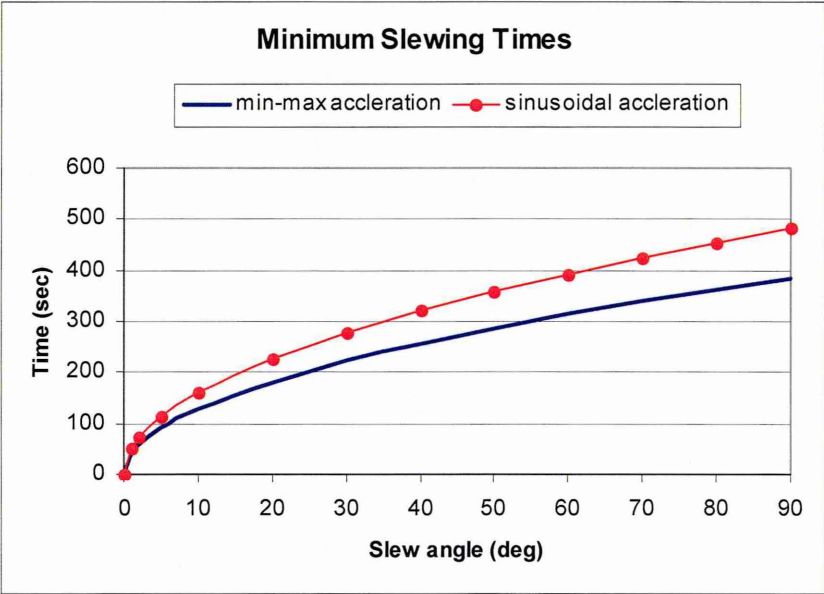
Figure 7-16 Minimum slew times in pitch axis ( T_{(max)} = 5 \mu\text{N.m} ; I = 0.1174 \text{ kg.m}^2 )
