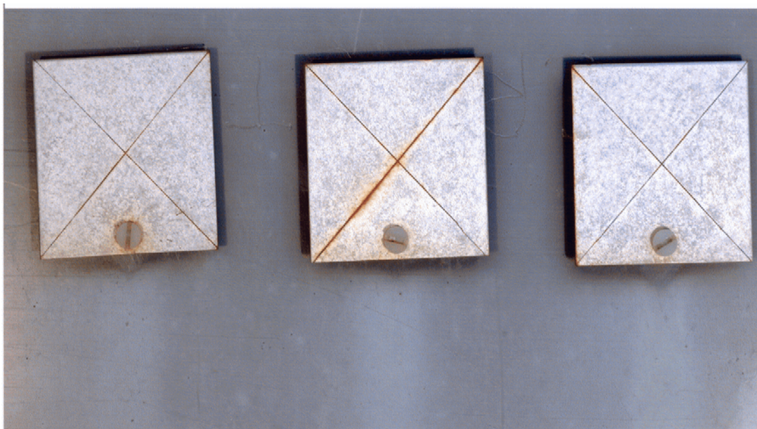
Figure 101. Scribed SermeTel coated panels after 12 months of marine atmosphere exposure
