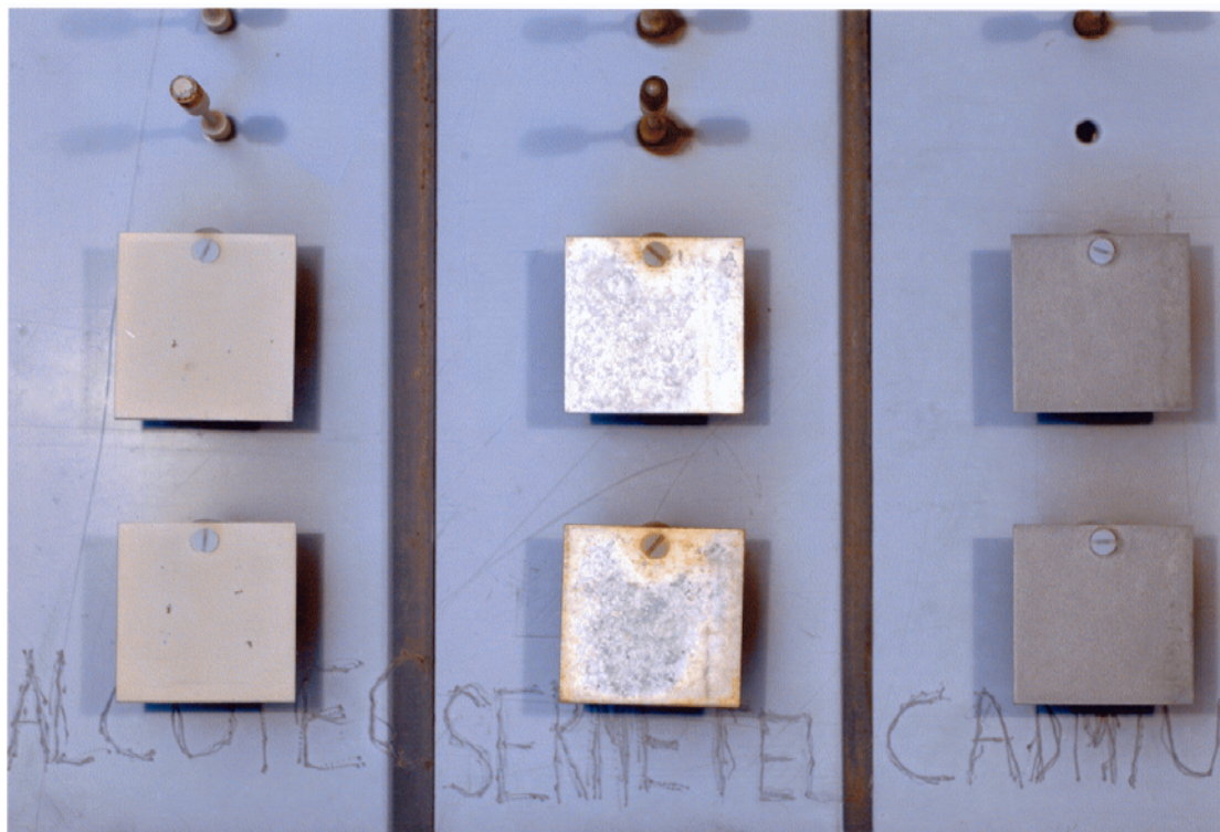
Figure 96. Unscribed coated panels exposed to marine atmosphere for 2 years
