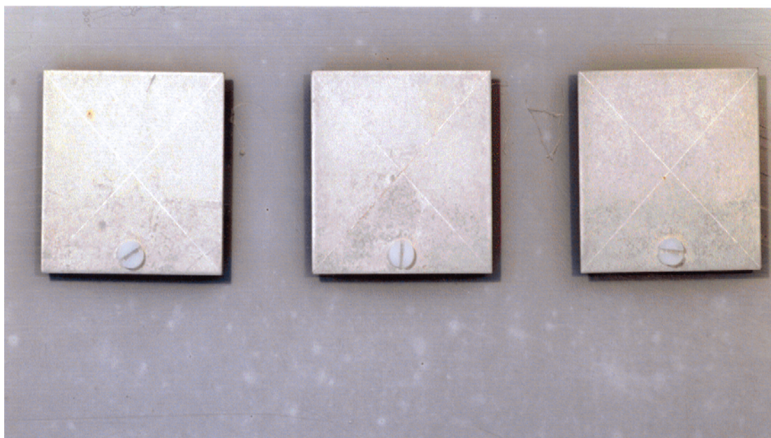
Figure 102. Scribed Cd coated panels after 12 months of marine atmosphere exposure
