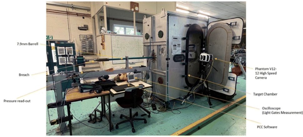
FIGURE 9 | ELVIS gas gun set up [59].
