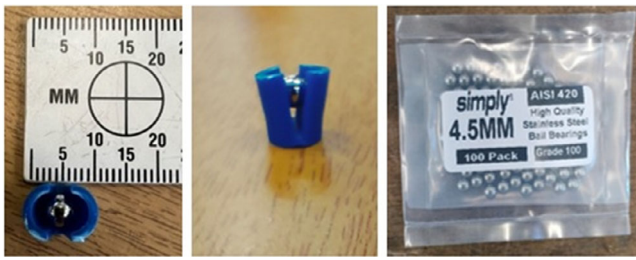
FIGURE 8 | 4.5 mm ball bearing inside plastic sabot.
