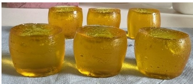
FIGURE 18 | Plastic deformation on Hartley's Jelly samples. Rear: Smooth face located on bottom platen. Front: Smooth face located on top platen.
