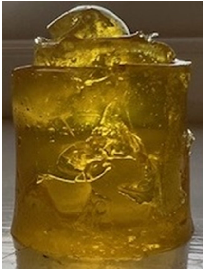
FIGURE 2 | 25 mm diameter Hartley's Jelly sample highlighting tearing to the outside surface during decanting.
