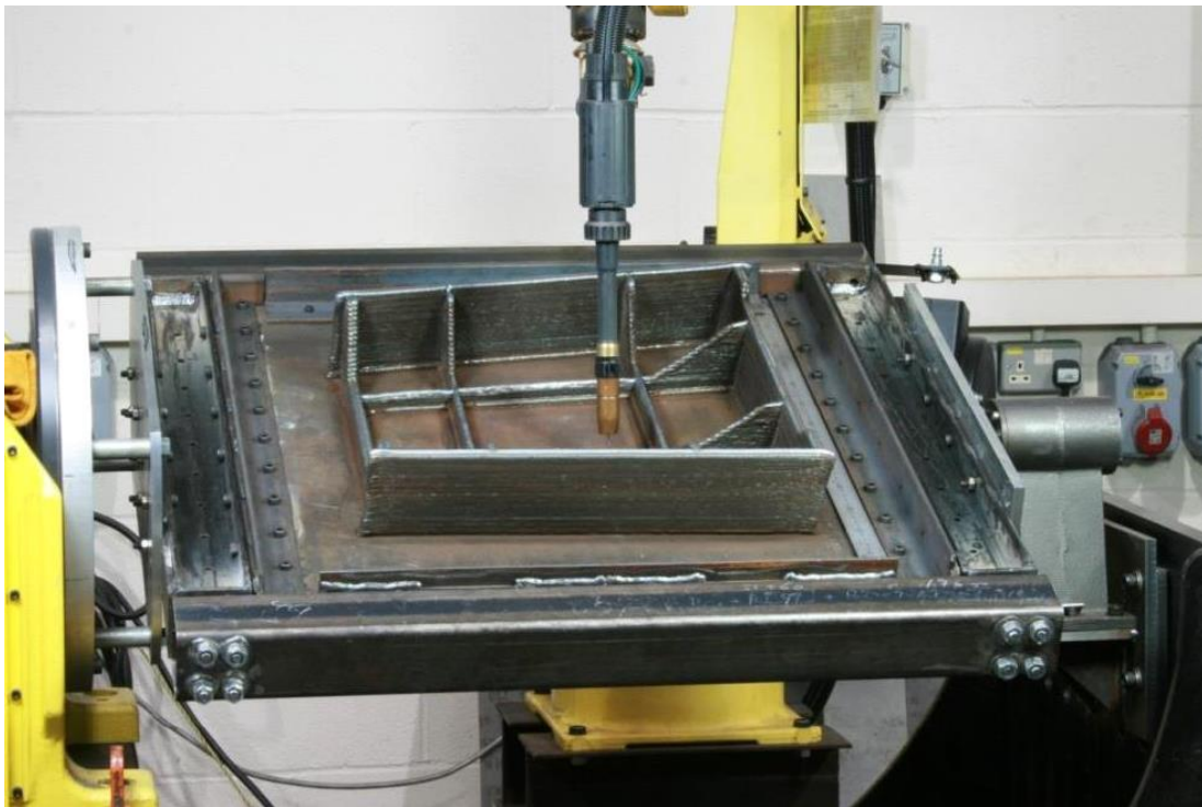
Figure 2-4 A GMA-based WAAM set-up for a complex large part [10].
