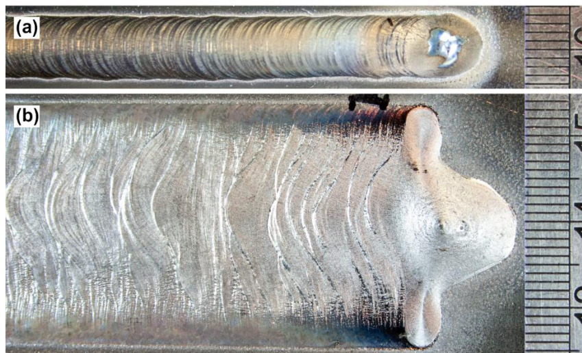
Figure 5-13 Comparison of the bead surface geometries: (a) PTA-only ( v_a = 0.5 mm/s), and (b) SL-reshaped ( v_a = 0.5 mm/s, w_s = 26.5 mm).
