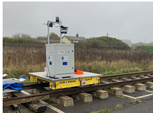
Figure 3.3: Converted RIMV with autonomous capability
