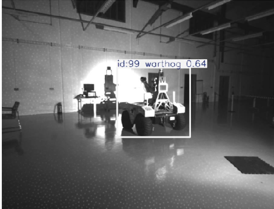
Figure 5.19: The confidence rate decreases with higher brightness at 1286 Lux
