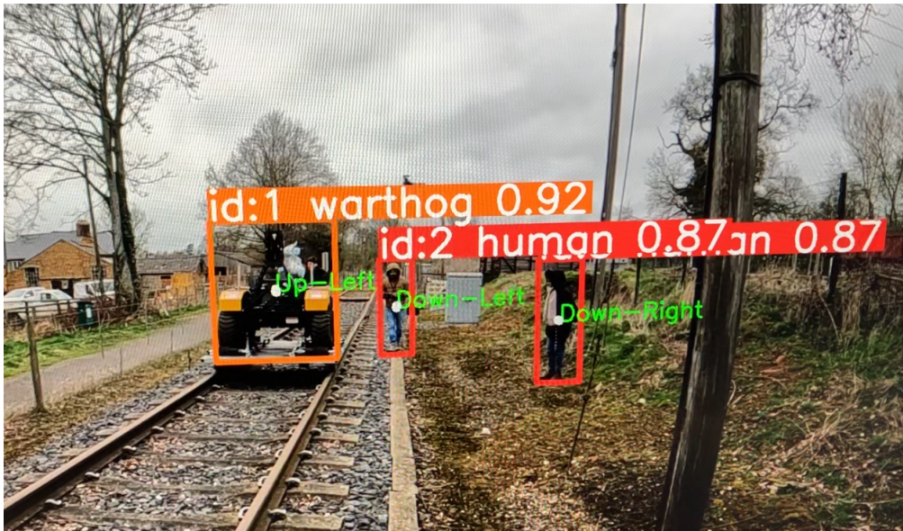
Figure 5.1: Example of 2D tracking result, the “warthog” vehicle refers to another type of autonomous railway robot used for maintenance tasks.
