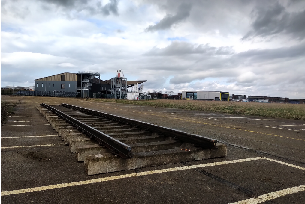
Figure 5.9: RITA contains a ballastless track with a standard track gauge of 1.435 metres and a total length of 18 metres, used for testing and validating autonomous railway systems.
