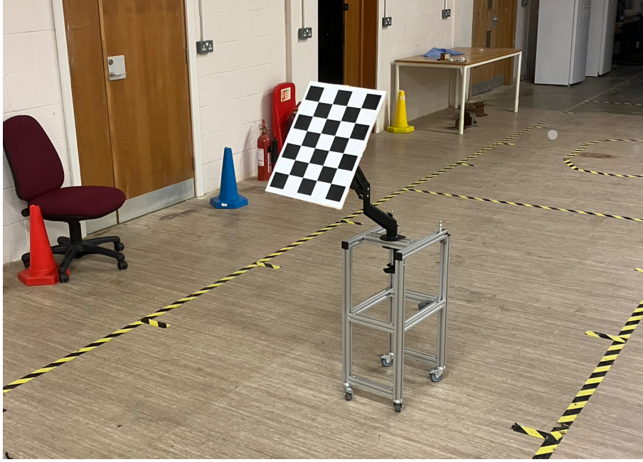
Figure 5.3: Chessboard used for camera LiDAR calibration
