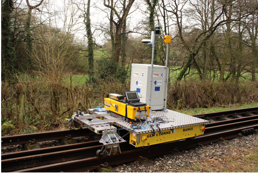
Figure 1.2: RIMV is a lightweight, adaptable, autonomous platform designed for railway maintenance tasks. Its modular design allows for integration with various equipment to suit different maintenance requirements. This image showcases the vehicle equipped with ultrasonic testing technology for rail defect detection on an active railway track under possession.
