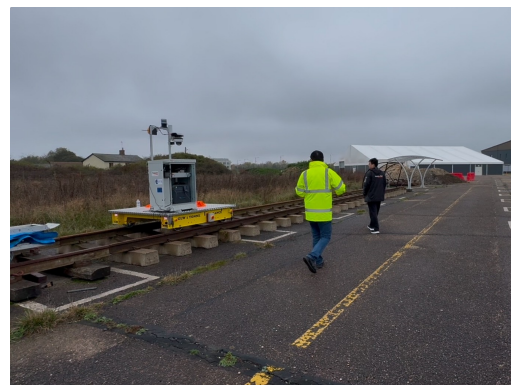
Figure 1.5: Outdoor collision avoidance validation with worker and trespasser
