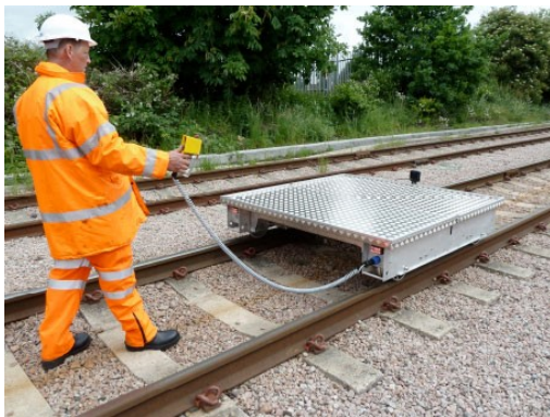
Figure 3.2: Original bance rail trolley with hand controller
