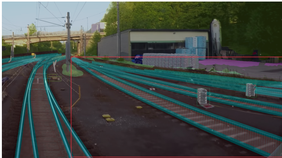
Figure 4.4: Comparison of polyline and bounding box annotation (where the teal line is the polyline representation, and the red line is the bounding box representation, better seen in colour).
