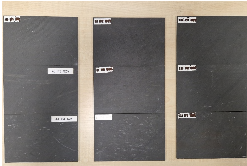
Figure 4-4 CFRP samples that have undergone impact damage at energies of 4J (left) 8J (middle) and 12J (right)
