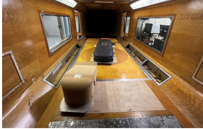
Fig. 2 Testing setup at Cranfield University 8x6 ft wind tunnel
