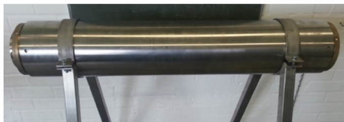
Fig. 2. Custom-made core holder for large-scale core-flooding experiments.
