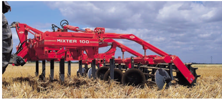
Figure 2. Tine stubble cultivator suitable for minimum tillage
