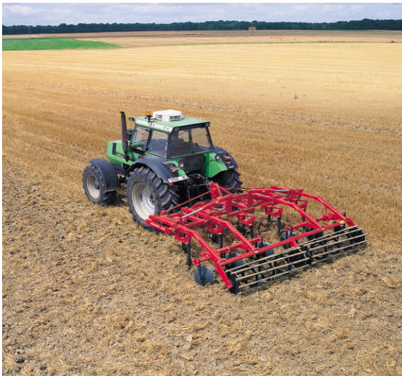
Figure 1. Two operations in traditional tillage system: stubble cultivation and ploughing
