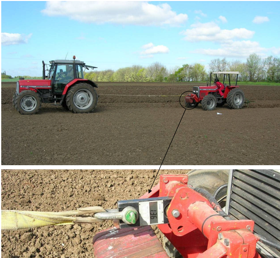
Figure 10. Location of the digital tension meter between the tractors and detail of the digital tension meter
